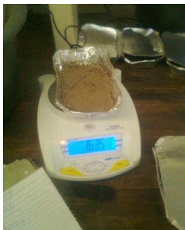
Figure 3: Soil sample on weighing balance (a) and soil samples in the oven (b).
