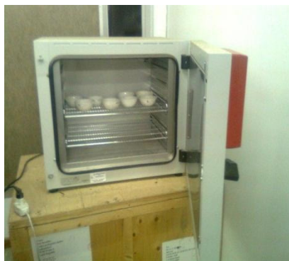
Figure 5: The soil samples in the oven after sedimentation was done.
