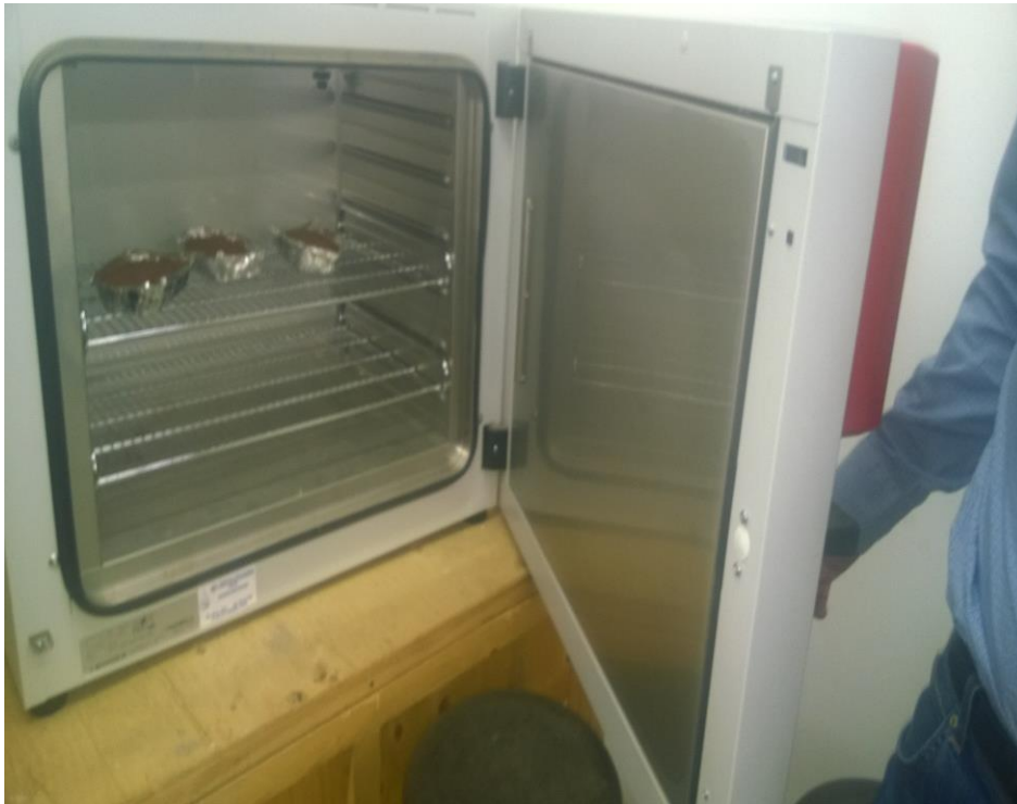
Figure 12: Drying Oven (Binder) for drying samples before sieving. (Photo taken by Reginalda, 2015)
