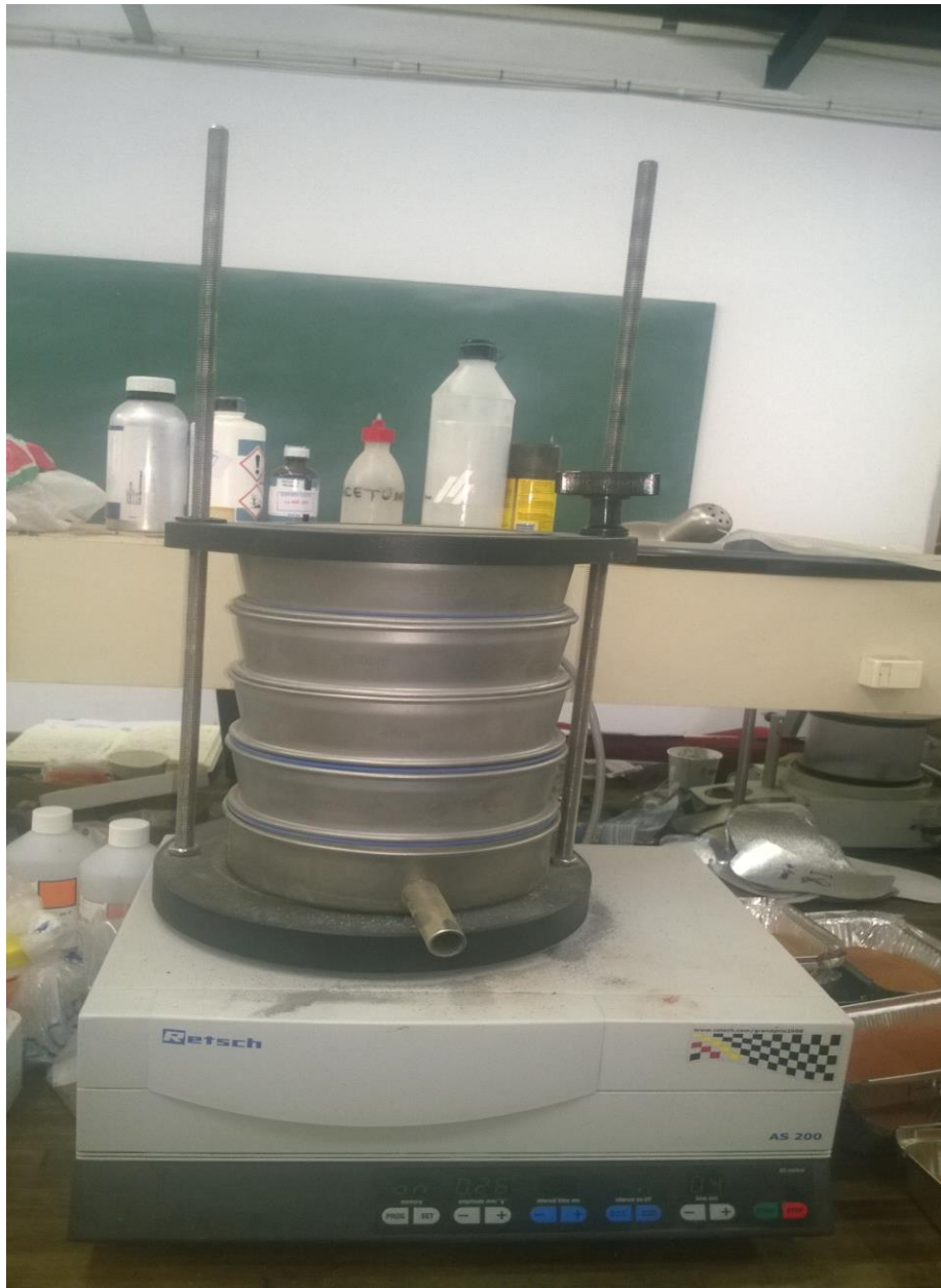
Figure 13: Sieves used for grain size analysis .The Retsch AS 200 sieve shake was used to facilitate the movement of sediment through the sieves (Photo taken by Reginalda, 2015).
