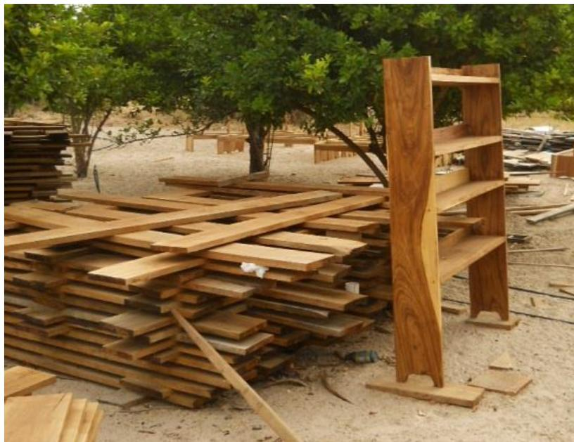
Figure 3: Kiaat *P. angolensis* planks showing the pale sapwood and the darker heartwood
