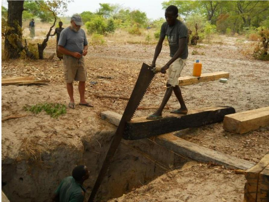
Figure 7: Pit sawing of Kiaat *Pterocarpus angolensis* logs
