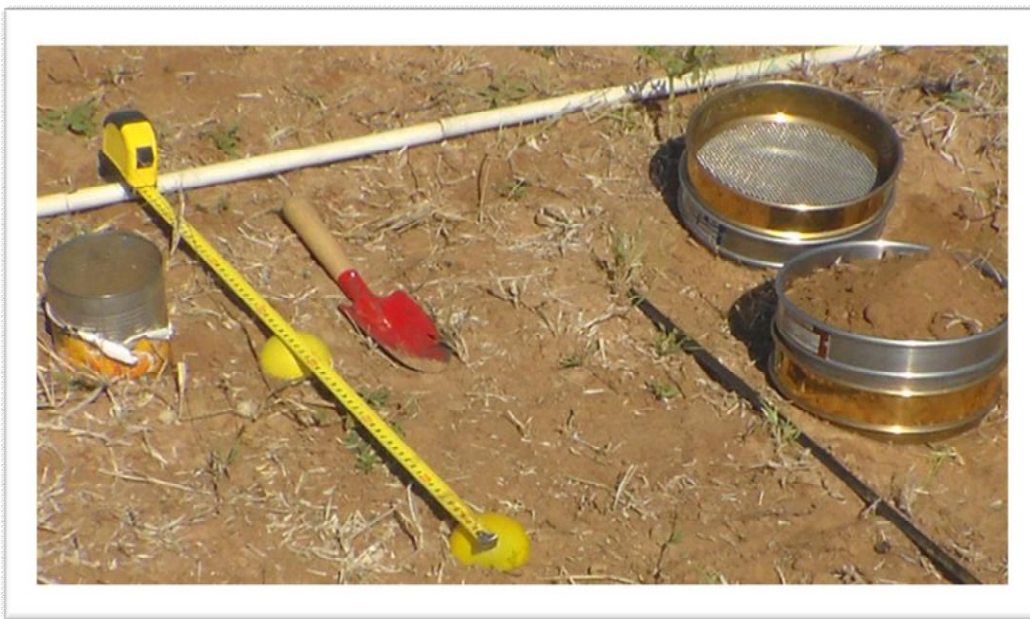
Figure 9: The tools used to collect soil seed bank data: 500g peach tin, a garden trowel, measuring tape and the yellow marker. The 2mm and 1mm sieves (placed on top of each with 1mm at the bottom) were used to recover the seeds from the sand.
