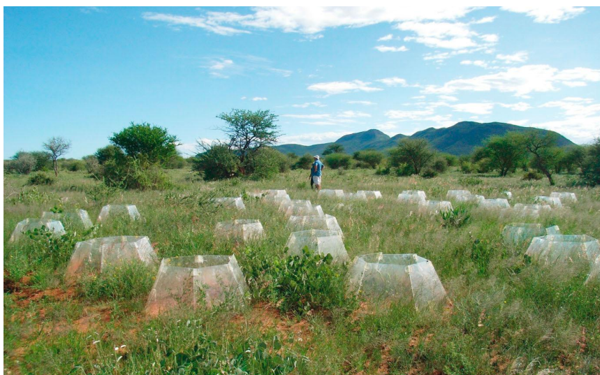
Figure 4: Open top chambers (OTC) on a bush-cleared site in the thornbush savanna in Namibia (Erichsfelde Farm).
