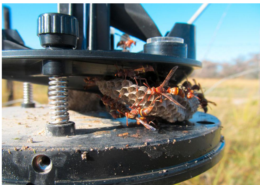
Figure 5: Wasps inside the sensor causing false rainfall values at Kalimbeza weather station.
