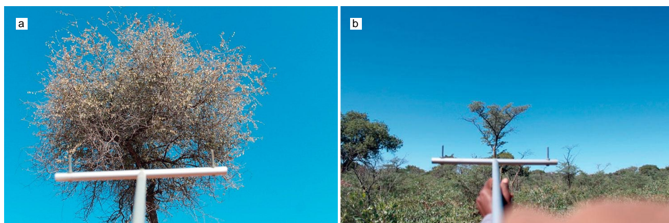
Figure 4: The use of the Bitterlich gauge (a) pointed at a woody canopy to estimate woody cover. In this instance, the overlap of the tree canopy past the pins means this is recorded as cover and (b) pointed at a woody canopy to estimate woody cover. In this instance, there is no overlap and thus this is not recorded as cover (Images: D.F Joubert, J.A.N Kandjai).
